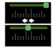
If the measurement is correct, the Next button appears. By pressing the button the printer proceed to the next measuring point. Once all three measurement points have been completed, the printer will re-check the distances.
